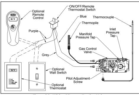
Figure 36. Wiring Diagram For Gas Valve.
